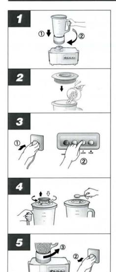
Attach the container and container base first and place it on motor housing. Twist container clockwise to lock.
