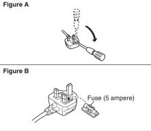
2. Replace the fuse and close or attach the fuse cover
